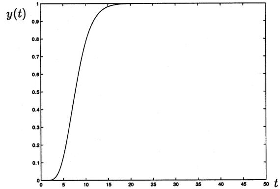
Fig. 6. Unit step response of  $G(s) = 1/(s + 1)^8$ .
