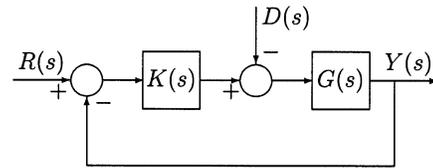
Fig. 3. Block diagram of a feedback control systems.
