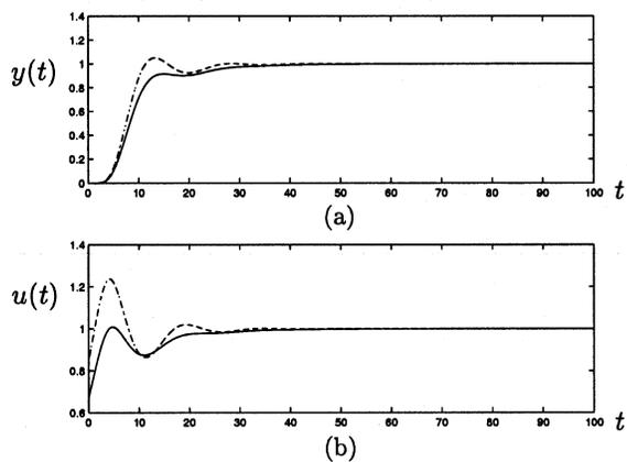
Fig. 9. (a) Step response and (b) control signal for the closed-loop system with PID controllers tuned by following the proposed methodology with  $K_p = 0.6699$  (solid lines) and  $K_p = 0.8460$  (dashed lines).
