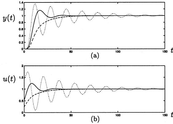
Fig. 7. (a) Step response and (b) control signal for the closed-loop system with the PI controllers of Table II. Ziegler–Nichols (dotted lines). Proposed methodology with  $K_p = 0.25$  (dashed lines).  $K_p = 0.5249$  (solid lines).
