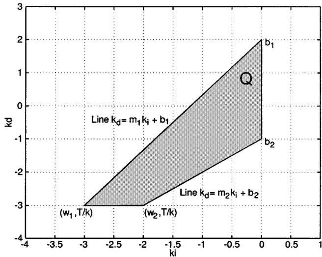
Fig. 4. The stabilizing region of  $(k_i, k_d)$  for  $k_t < k_p < -(1/k)$ .
