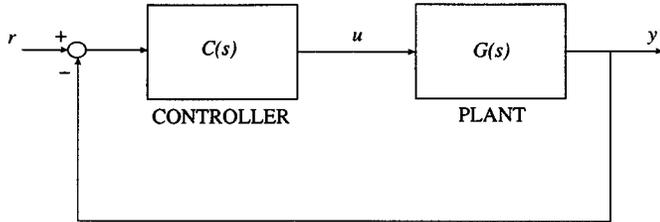
Fig. 2. Feedback control system.
