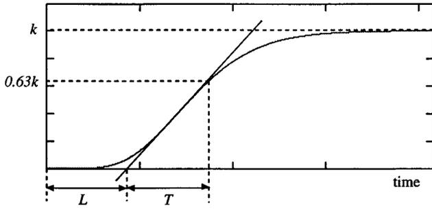
Fig. 1. Open-loop step response.
