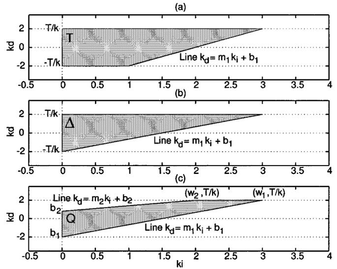
Fig. 3. The stabilizing region of  $(k_i, k_d)$  for: (a)  $-1/k < k_p < 1/k$ . (b)  $k_p = 1/k$ . (c)  $1/k < k_p < k_u$ .
